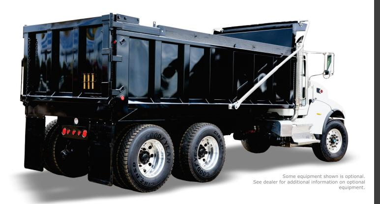
FEATURES VERTICAL SIDE BRACING AND RUGGED TOP RAILING CONTINUOUSLY WELDED FOR MAXIMUM STRENGTH
